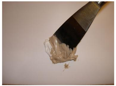
STEP 3. Mix and amalgamate the two components properly with either a putty knife or similar, make sure the hardener is mixed through thoroughly to ensure a even setting.
